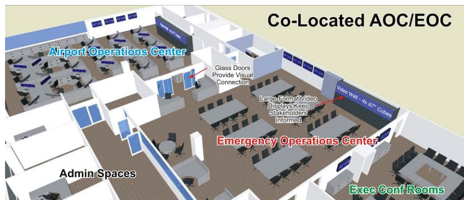
Figure 11: 3-D Model of SDI Command Center showing layout of Co-Located Airport Operations Center (AOC) and Emergency Operations Center (EOC).
