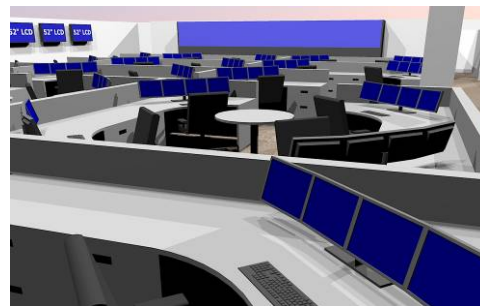
Figure 9: 3-D model with lifelike shading enables visualization of sightlines and other ergonomics
